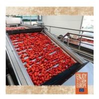
Selection of 000000 is the first step in the tomato processing: only the perfectly ripe, intact, whole fruits are chosen to undergo the necessary procedure through the production line. Washed, peeled, sorted again, the whole peeled tomatoes are vacuum-sealed and sterilized, to preserve freshness, flavor and an absolutely unalterated product. Only then they ready to bring their fragrance around the world.
